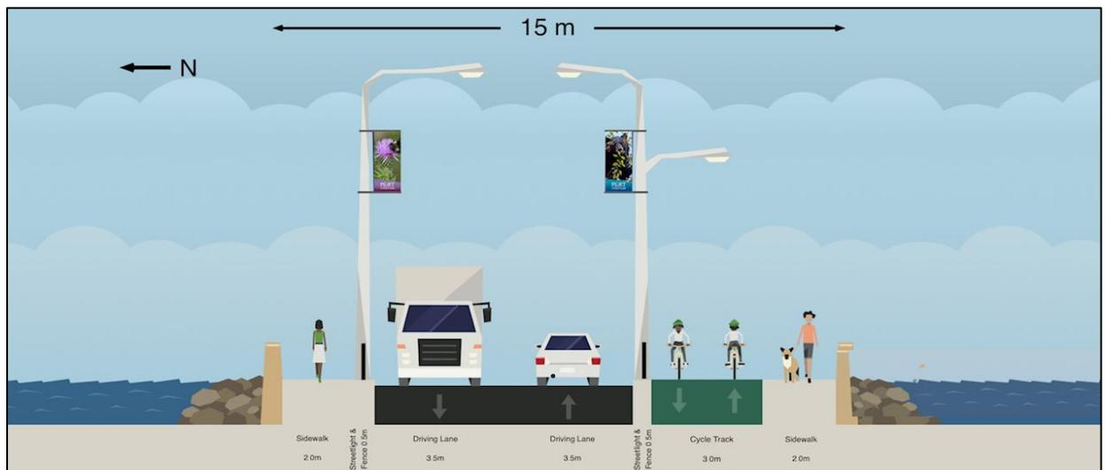
**Figure 10.3c Lincoln Connector Bridge Typical Cross Section**
