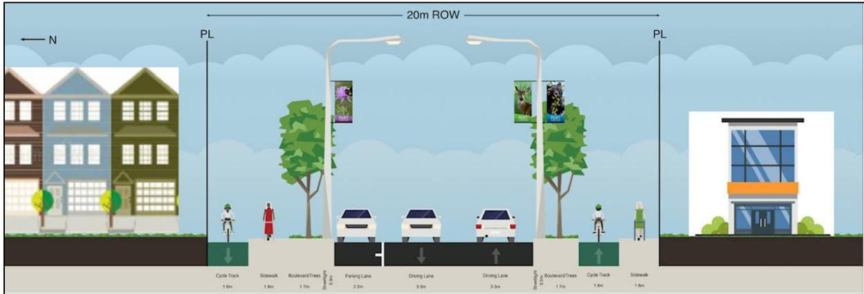
**Figure 9.1d: Dominion Avenue Streetscape - Typical Cross Section**
