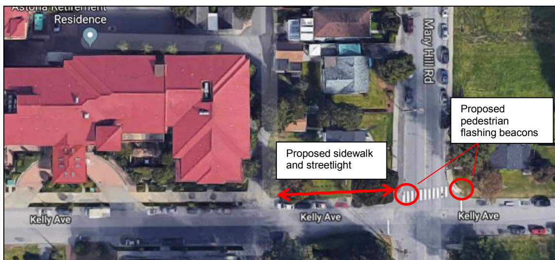
Figure 5: Kelly Avenue – sidewalk, streetlight and pedestrian flashing beacons
