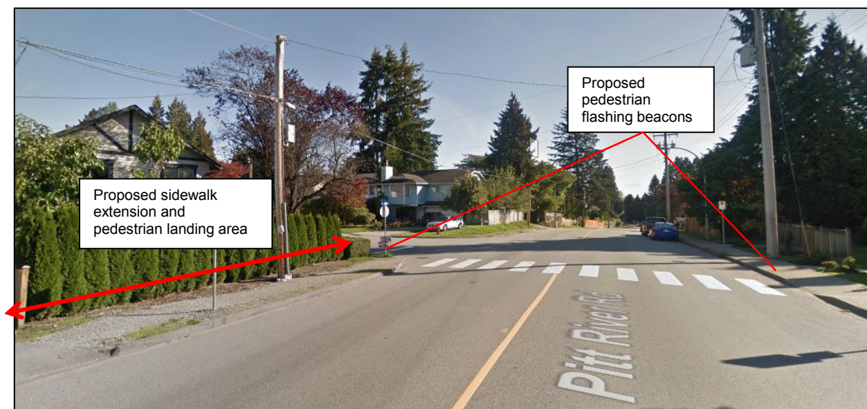
Figure 8: Pitt River Road at Yukon – proposed sidewalk and crosswalk improvements
