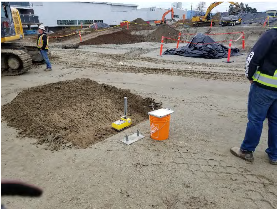
Photo 1 – Compaction testing of fill placed on November 14, 2019 (Item 3). [photo taken by JAL and dated 20191118]
