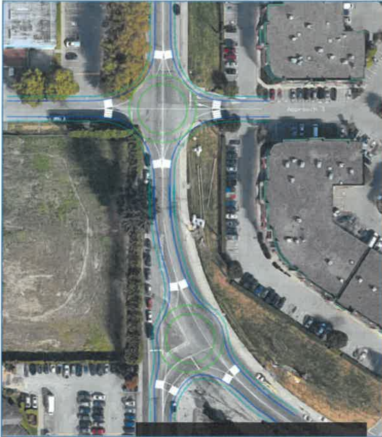
Figure 15: Roundabout layout at Kelly Ave and Tyner St at Kingsway
