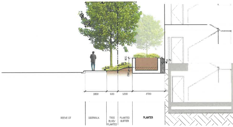
1 12.02 1:50 Ground Floor Section at Reeve Street
