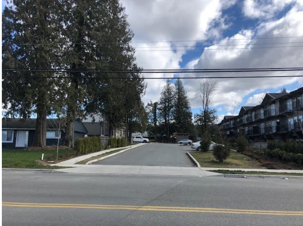
Example of new road and sidewalk well within critical root zone of neighboring trees. Tree show no signs of decline after 3 years.
