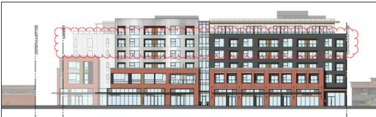
McAllister Avenue facade (with additional floor)
