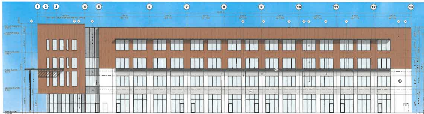
1 SOUTH ELEVATION (FACING SEABORNE AVE.) SCALE: 5/32" = 1'-0"
