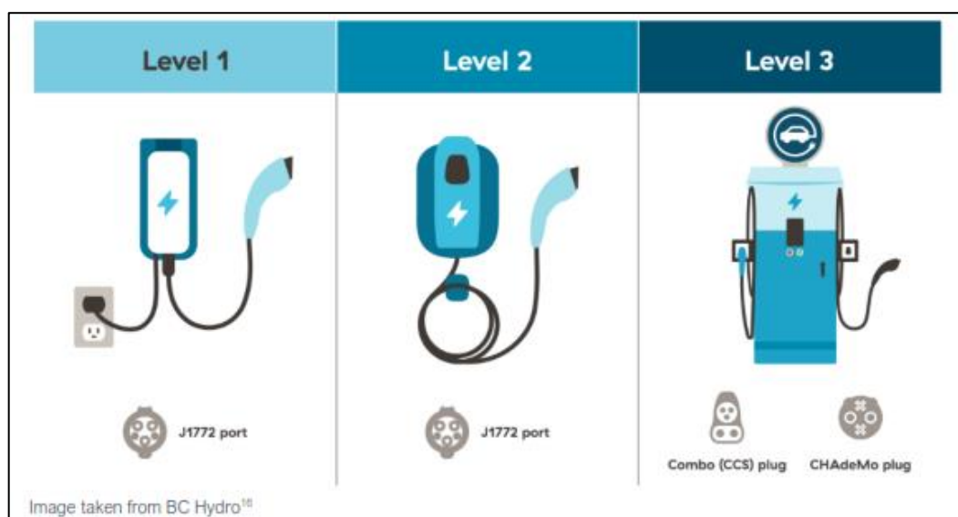
Figure 12.5: Level 1, 2 and 3 Charging Types
