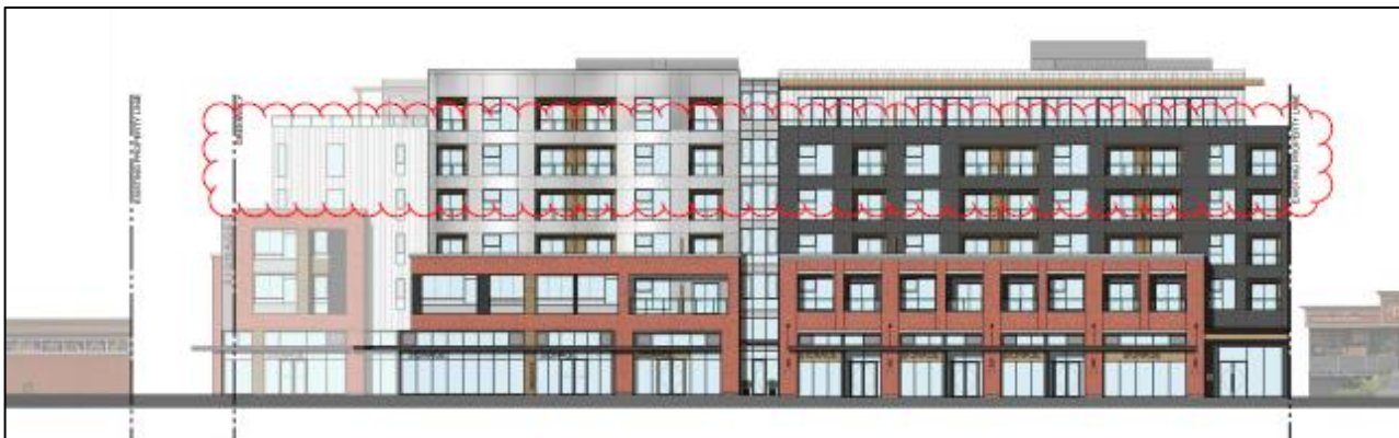
McAllister Avenue facade (with additional floor)
